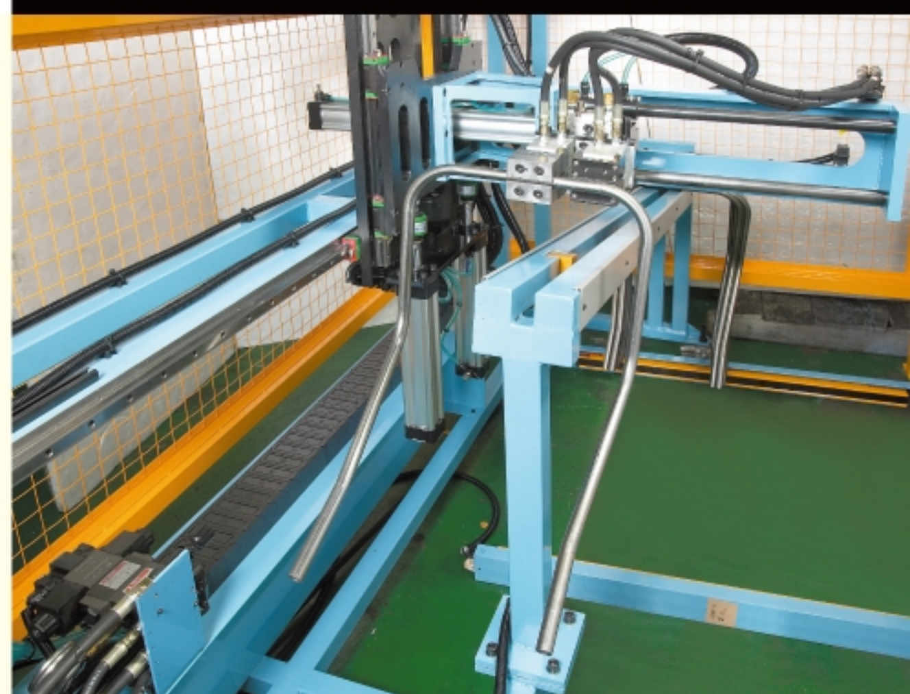
Automatic Unloading System ( AUL )
