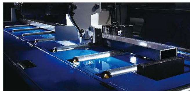
Electric Servo Controlled Feeding B
